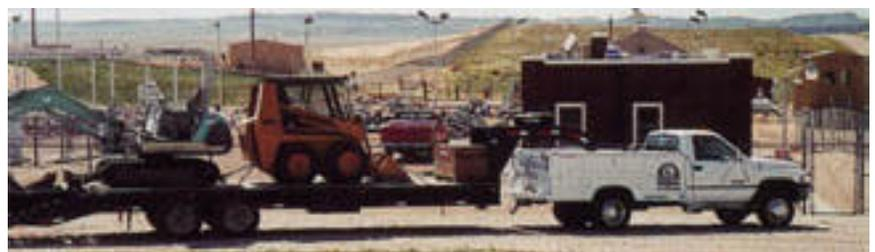
In addition to its efficiency on the job, small equipment is easier to transport. Pickup easily hauls trailer carrying mini-excavator, skid-steer loader and tool box.
