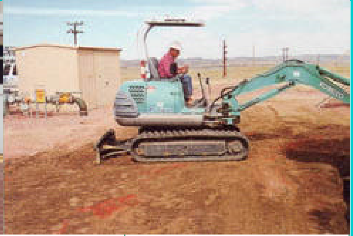
Jerry Long uses one of the Kobelco SK35s to dig a trench alongside a pumphouse at Guernsey. Zero tailswing of the diminutive excavator allows it to work right beside the structure.
