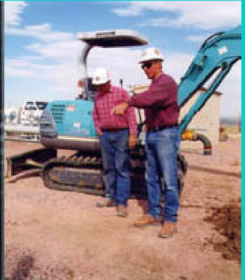
Another advantage of the miniexcavators: they can fit through doorways, facilitating excavation work inside buildings, as here at Platte Pipe Lines Moorefield, Neb., station, where lines serving the unit pumps had to be uncovered and reset.
